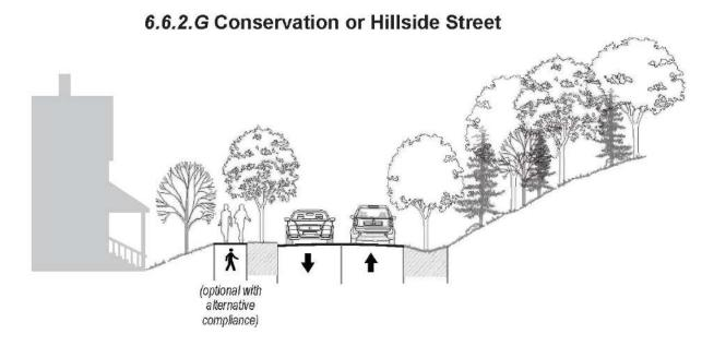
Definition: Streets designed to accommodate environmental constraints and to encourage minimal grading and adaption to the natural character of the land. This street standard can be applied when environmental issues, environmental protection and/ or conservation are a consideration. This standard can **only** be used with the pre-approval of the administrator.
