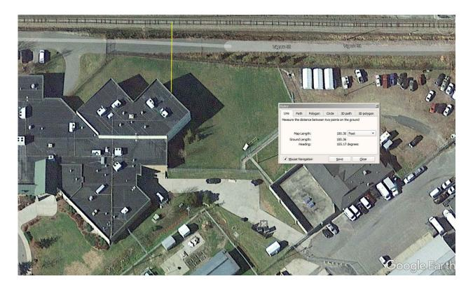
Using the ruler feature of Google Earth, I created a line from the center of the railroad tracks to the portion of the jail, a distance of 100 feet. Notice that the current jail encroaches the railroad right of way.
